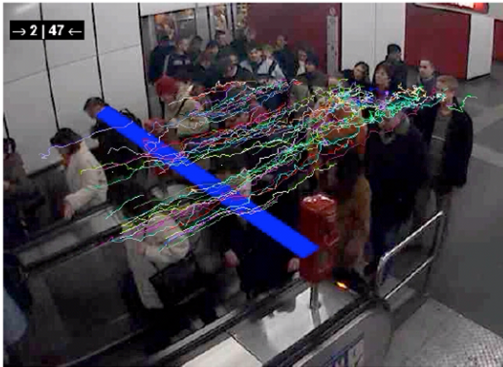
Figure 1. Crowded Scene in an Underground Station. Pedestrians which cross the bright (blue) line at the foot of the elevator are being counted in this scenario.
